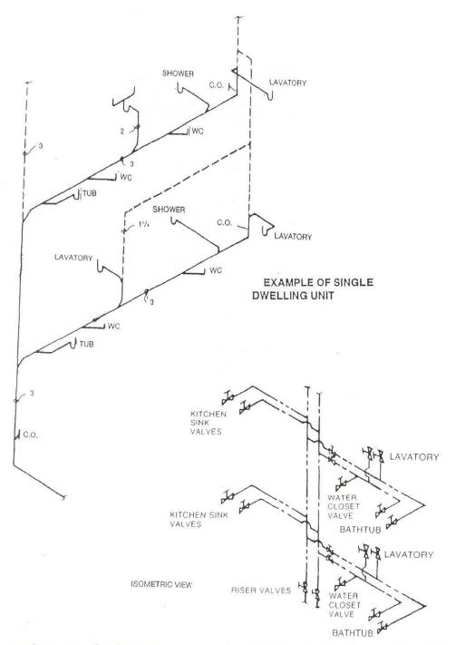
Whenever new water or drain lines are to be installed, a plumbing riser diagram is required. A plumbing riser diagram consists of water, drain and vent lines being installed. Indicate all pipe sizes and show cleanouts for the sanitary system. A sample of what a riser diagram consists of is shown above.
