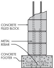
Homes must be anchored to resist flotation, collapse, and lateral movement by being tied down in accordance with your community's ordinance or the manufacturers' installation specifications for SFHAs.
