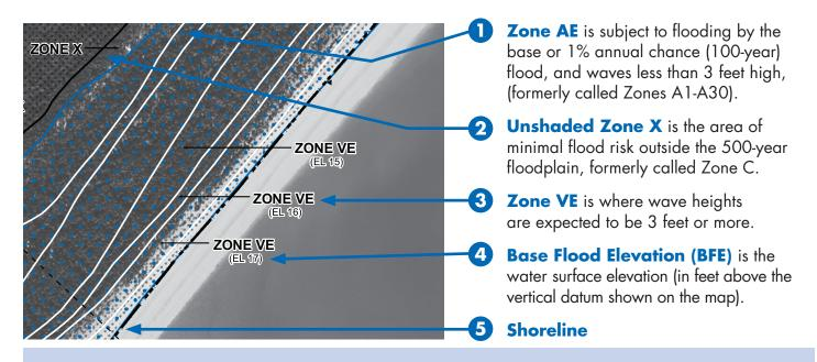
Some FIRMs published after 2009 may show the Limit of Moderate Wave Action (LiMWA). The LiMWA delineates where wave heights are less than 1.5 feet. The area between the LiMWA and the Zone V boundary is called the Coastal A Zone (see pages 15 and 16).
