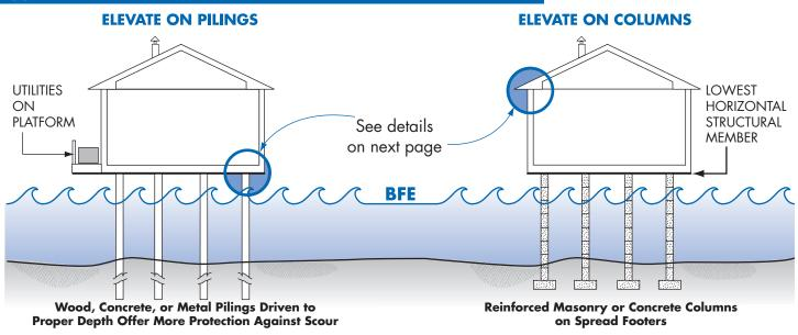
In Zone V, the design specifics will be determined by an architect or engineer based on the site, including how the building will be elevated and how deep the foundation elements will be in the ground.
