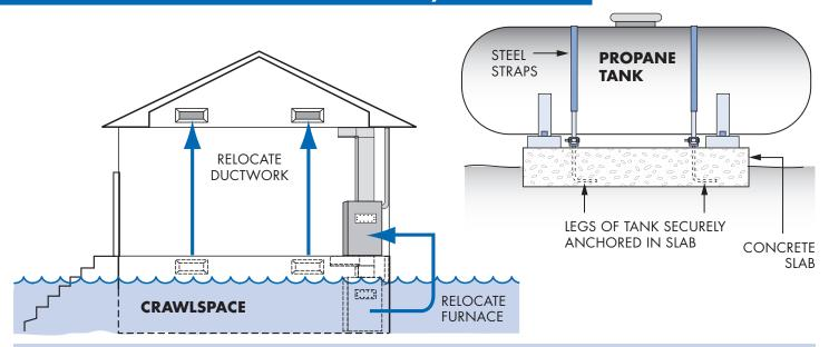
Move fuse boxes, water heaters, furnaces, and ductwork out of crawlspaces and basements.
