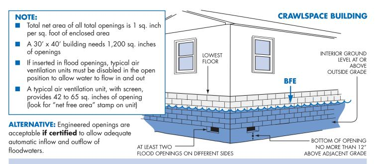
Solid perimeter wall foundations can enclose flood-prone space. A crawlspace is a good way to elevate just a couple of feet. In all cases, the following are required: flood openings, elevated utilities, flood-resistant materials, and limitations on use.
