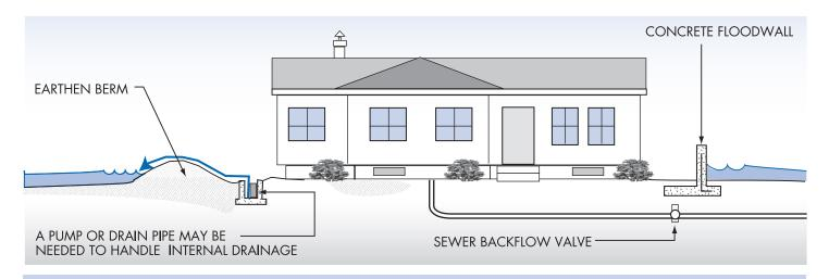
In areas where floodwaters aren't expected to be deep, sometimes individual buildings can be protected by earthen berms or concrete floodwalls. Permits are required for these protection measures and extra care must be taken if the site is in a floodway (see page 33). A small berm or floodwall does not remove elevation requirements and cannot be use to achieve compliance for a new or substantially improved building, or one that is repaired after substantial damage.
