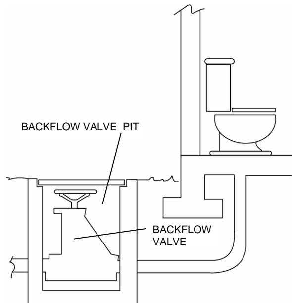
← NORMAL DIRECTION OF FLOW (VALVE PREVENTS FLOW IN REVERSE DIRECTION)
